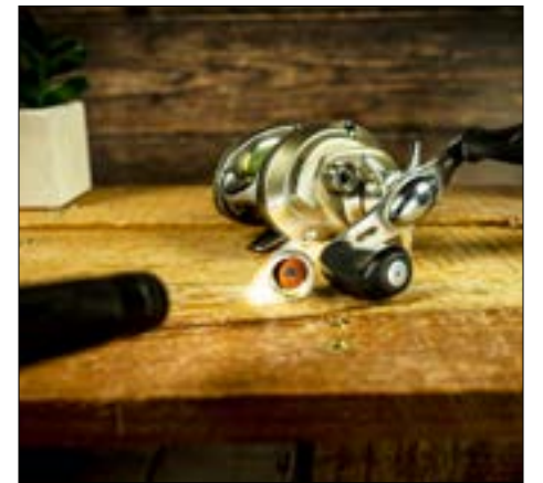
A flashlight helps show the old grimy oil deposit in the tension knob. Wipe it out and start fresh with just a single drop of oil.
