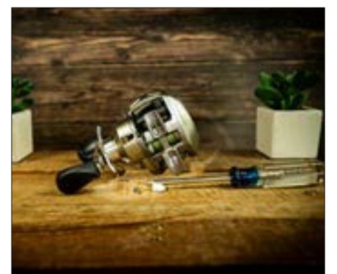
Removing the 'trap door' covering the underside grease port allows easy access to the main drive gear. Apply grease here if possible.
