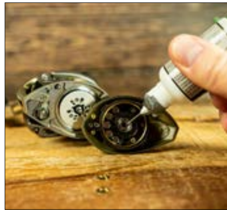
The side plate bearing is an important place to oil; so is the brake ring—if one is present on your reel.
